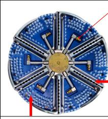
Name: 4 - 6pcs 0-500PSI spray jets .Working: The pressure vapor water spray out by 0-500PSI working pressure to the bottom of the carpet to clean the dust or chemical-left. FPM: 6L
